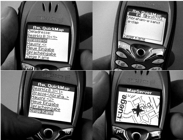
Figure 2. GUI-only map selection in the QuickMap WAP page: in the example, at least 60 key-presses are required before the map is displayed, including 44 key-presses just for entering the lengthy street name “Abraham-a-Sancta-Clara-G” (compare figure 3).
