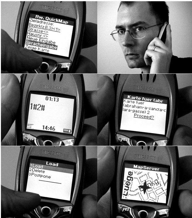
Figure 3. Multi-modal or voice-only address entry in the QuickMap demonstrator. The user can initiate the voice call to the dialog system either directly or through the WAP page. DTMF can be used during the dialog for safe entry of numeric form-field values (district and street number, third picture). When the voice-form is complete, the application server requests the network to send a WAP-Push message to the mobile phone. The WAP-Push message seizes control of the display (fourth picture). After selecting Proceed, the T68 phone asks the user whether to load the document linked in the WAP-Push message through a GPRS connection.
